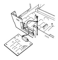
2. Holding the interface board level, rotate it clockwise into position and **attach** it to the main board. Make sure the connector pins are properly inserted into the mating connector.
